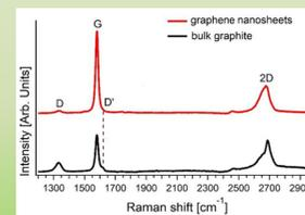
Moreover, the  $I_D/I_G$  ratio as low as 0.07±0.01 in graphene Raman spectra evidences the very low amount of defect induced by exfoliation.
