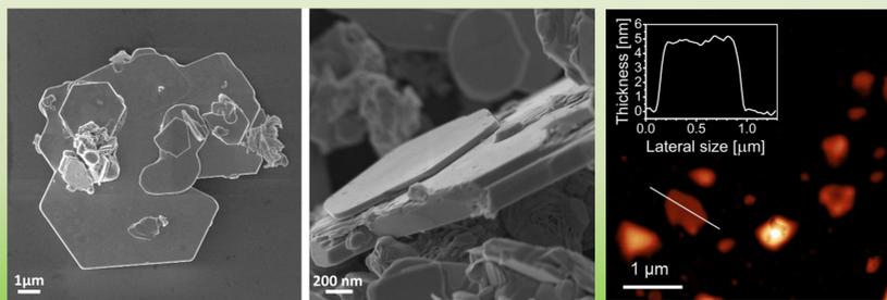
collected along the with line, allow concluding that Polarclean-assisted LPE provides flakes with an aspect ratio of ~10<sup>3</sup>.
