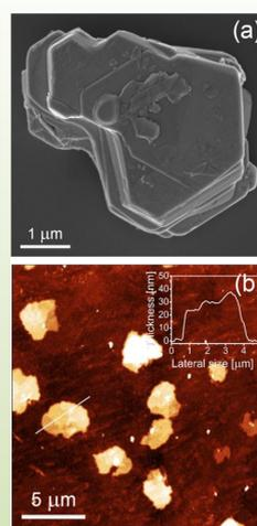
The procedure was extended also to MoS<sub>2</sub> and graphene. Regarding MoS<sub>2</sub>, statistics reveal results comparable with that of WS<sub>2</sub>. For graphene, remarkably the distribution of lateral size shows an average value of 10 μm, which is one of the largest ever reported for LPE.
