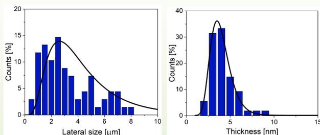
Statistical analysis of lateral size and thickness of WS<sub>2</sub> flakes based on SEM and AFM images demonstrate that lateral size and thickness of the flakes approximately follow log-normal distribution peaked at ~3 μm and ~4 nm respectively.
