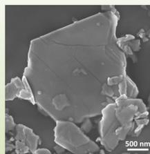
The formation of the SnO<sub>2</sub> surface oxide layer was demonstrated with several surface science techniques. In particular, the analysis of XPS spectra allowed to estimate the thickness of such layer which is calculated to be equal to 8 ± 1 Å, without noticeable changes after aging in air in a time scale of 1 week [1].
