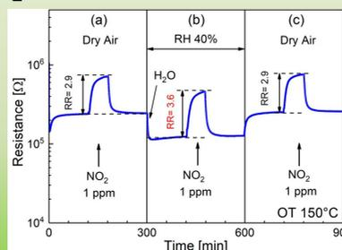
Reproducibility test over a period of six months of continuous operation at 150°C demonstrated remarkable long-term stability of the electrical properties including NO<sub>2</sub> and H<sub>2</sub> response.
