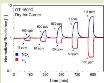
The SnO<sub>2</sub>/SnSe<sub>2</sub> heterostructure demonstrated comparable response as that of layered TMDCs (resistance ratio = 3.2 to 1 ppm NO<sub>2</sub>) and first experimental evidence ultrahigh response to H<sub>2</sub> at 150°C among the best measured to date for TMDCs based H<sub>2</sub> sensors.
