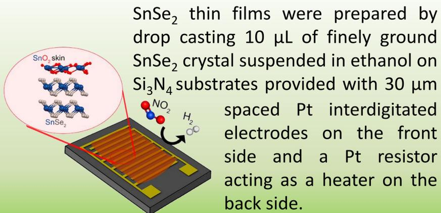
SnSe<sub>2</sub> thin films were prepared by drop casting 10 μL of finely ground SnSe<sub>2</sub> crystal suspended in ethanol on Si<sub>3</sub>N<sub>4</sub> substrates provided with 30 μm spaced Pt interdigitated electrodes on the front side and a Pt resistor acting as a heater on the back side.
