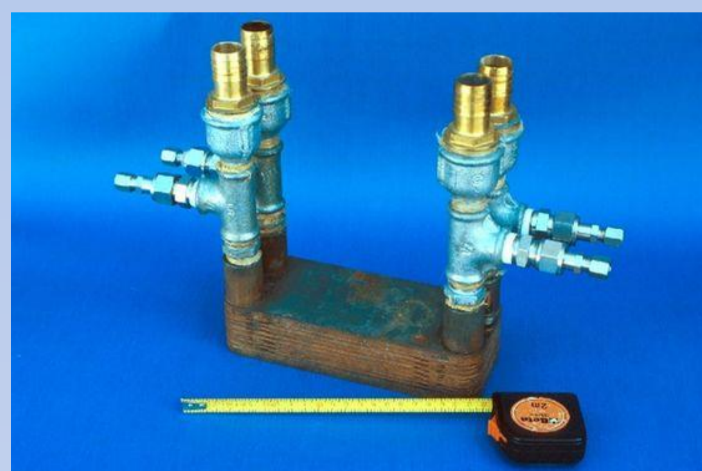
Heat exchanger for absorption machines realized in ENEA .
