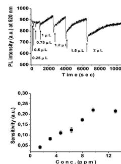
The photoluminescence of the composite when exposed to green light (520 nm) decreased proportionally to the concentration of acetic acid to which it was exposed.
