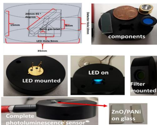
We developed a sensor based on photoluminescence transduction. A thin layer of ZnO/PANI composite deposited on a glass substrate showed remarkable sensitivity to acetic acid.
