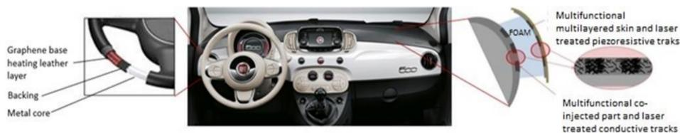
The most challenging effort will be finding and testing all polymeric matrices of the dashboard in order to find a proper GRM concentrations for each polymer that shows conductivity and piezoresistivity only after the LISA process. The main functionality that this technology could replace will be the pressure sensors (switches and knobs) and the electrical circuit for the stirring wheel electric heating.
