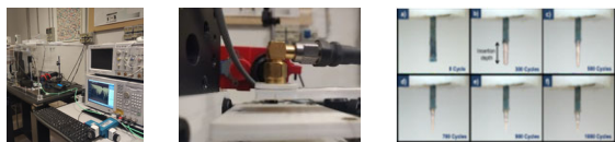
Fig.2 – Scanning Near Field Microscopy setup: VNA Agilent E5071B (300 KHz to 8.5 GHz), SMA connector with etched tip and 3D printed chuck and sample holder.
