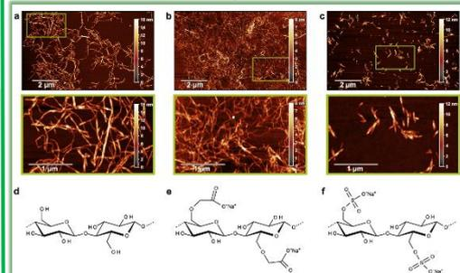
Fig.8 AFM images of: (a)(CNF); (b)(CCNF); (c)(CNC), and the corresponding simplified surface chemistries (d-f).
