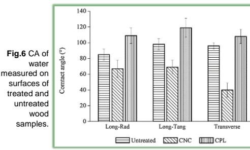
Fig.6 CA of water measured on surfaces of treated and untreated wood samples.
