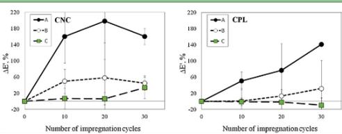
Fig.5 ΔE' vs. number of impregnation cycles for the two consolidants CNC and CPL on wood samples of different decay classes.
