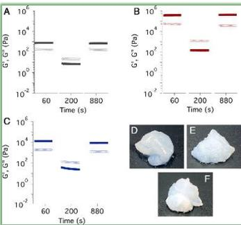
Fig.2 3ITT of GC (A), GC-OH<sub>3</sub> (B) and GC-CO<sub>3</sub> (C); the visual aspect of the samples: GC (D), GC-OH<sub>3</sub> (E) and GC-CO<sub>3</sub> (F).
