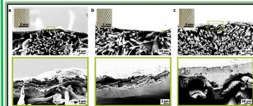
Fig.9 SEM images of aged cotton canvases coated 3 times with: (a) CNF; (b) CCNF and (c) CNC, with OM images as insets (left top).
