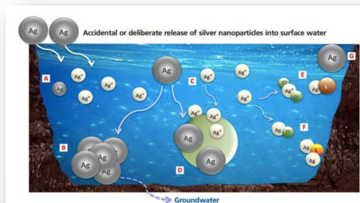
Figure 1. (A) Dissolution process leading to free ions release and smaller particles; (B) Aggregation into larger particles; (C, D) Adsorption of released Ag + and nAg, respectively; (E) Formation of soluble complexes; (F) Reaction with other components in the water, which may result in precipitation; (G) nAg remaining stable.
