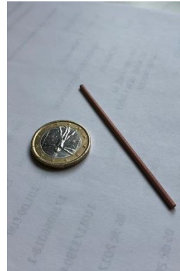
Specimen dimensions \phi = 2\text{mm} , h = 60\text{mm}
